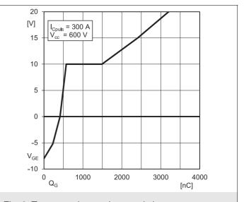
Fig. 6: Typ. gate charge characteristic
