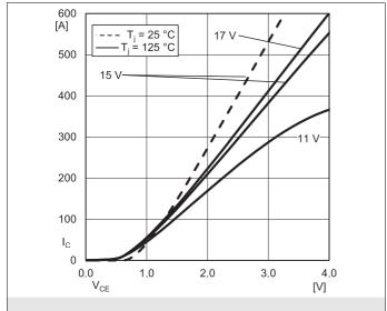
Fig. 1: Typ. output characteristic, inclusive  $R_{CC'+\; EE'}$
