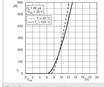
Fig. 5: Typ. transfer characteristic
